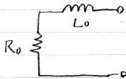
$$Y_0 = \frac{1}{R_0 + j\omega L_0} = \frac{R_0 - j\omega L_0}{R_0^2 + \omega^2 L_0^2} = G + jB$$
