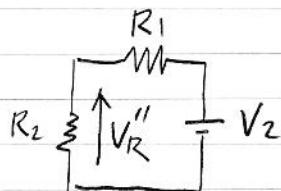
$$V_R'' = \frac{R_2}{R_1 + R_2} V_2$$
