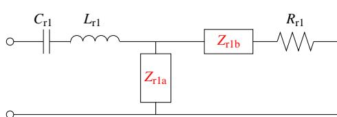
$$C_{r1} = \frac{L_1}{R_0^2}, \quad L_{r1} = C_1 R_0^2, \quad R_{r1} = \frac{R_0^2}{R_1}$$
