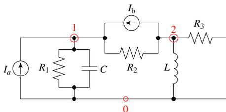
$$\begin{bmatrix} I_a + I_b \\ -I_b \end{bmatrix} = \begin{bmatrix} \frac{1}{R_1} + \frac{1}{R_2} + j\omega C & -\frac{1}{R_2} \\ -\frac{1}{R_2} & \frac{1}{R_2} + \frac{1}{R_3} + \frac{1}{j\omega L} \end{bmatrix} \begin{bmatrix} V_1 \\ V_2 \end{bmatrix}$$
