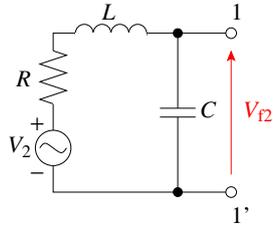
$$V_{f2} = \frac{\frac{1}{j\omega C}}{R + j\omega L + \frac{1}{j\omega C}} \cdot V_2 = \frac{-j5}{5 + j5 - j5} \cdot 5 = -j5 \text{ V}$$
