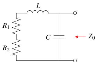
$$\begin{aligned} Y_0 &= \frac{1}{R_1 + R_2 + j\omega L} + j\omega C \\ &= \frac{1}{3 + j4} + j = \frac{3 - j4}{3^2 + 4^2} + j = \frac{3 - j4}{25} + j = \frac{3 - j4}{25} + j \frac{25}{25} = \frac{3 + j21}{25} \\ &= \frac{3(1 + j7)}{25} \text{ S} \end{aligned}$$
