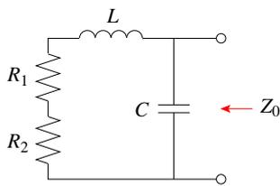
$$\begin{aligned} Z_0 &= (R_1 + R_2 + j\omega L) // \frac{1}{j\omega C} = \frac{(R_1 + R_2 + j\omega L) \cdot \frac{1}{j\omega C}}{(R_1 + R_2 + j\omega L) + \frac{1}{j\omega C}} \\ &= \frac{R_1 + R_2 + j\omega L}{(1 - \omega^2 CL) + j\omega C(R_1 + R_2)} \\ &= \frac{3 + j4}{-3 + j3} = \frac{(3 + j4)(-3 - j3)}{(-3)^2 + 3^2} = \frac{3 - j21}{18} = \frac{1 - j7}{6} \Omega \end{aligned}$$
