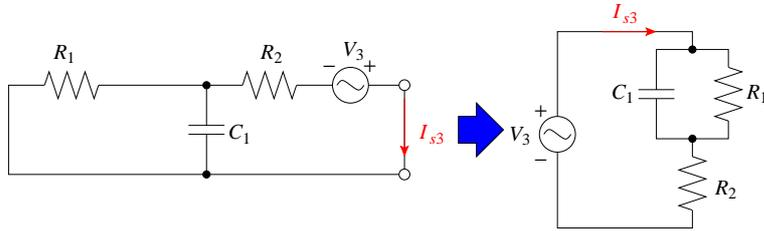
$$I_{s3} = \frac{V_3}{R_2 + \left( R_1 // \frac{1}{j\omega C} \right)} = \frac{V_3}{R_2 + \frac{\frac{R_1}{j\omega C_1}}{R_1 + \frac{1}{j\omega C_1}}} = \frac{(1 + j\omega C_1 R_1) V_3}{R_1 + R_2 + j\omega C_1 R_1 R_2}$$
