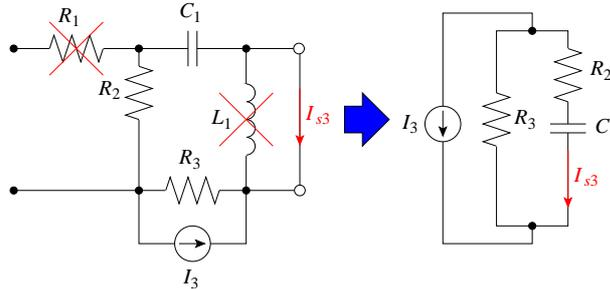
$$\begin{aligned} I_{s3} &= \frac{R_3}{R_3 + \left(R_2 + \frac{1}{j\omega C_1}\right)} (-I_3) = \frac{-j\omega C_1 R_3 I_3}{1 + j\omega C_1(R_2 + R_3)} \\ &= \frac{-j10}{1 + j4} = \frac{-10(4 + j)}{17} \text{ V} \end{aligned}$$
