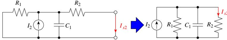
$$I_{s2} = \frac{\frac{1}{R_2}}{\frac{1}{R_1} + \frac{1}{R_2} + j\omega C_1} I_2 = \frac{R_1 I_2}{R_1 + R_2 + j\omega C_1 R_1 R_2} = \frac{5}{2 + j2} = \frac{5}{4}(1 - j) \text{ A}$$
