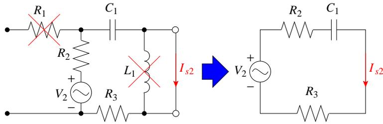
$$I_{s2} = \frac{V_2}{R_2 + R_3 + \frac{1}{j\omega C_1}} = \frac{j\omega C_1 V_2}{1 + j\omega C_1(R_2 + R_3)} = \frac{j20}{1 + j4} = \frac{20(4 + j)}{17} \text{ A}$$
