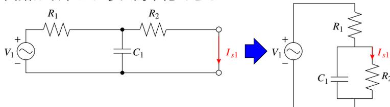
$$I_{s1} = \frac{V_1}{R_1 + \left(R_2 // \frac{1}{j\omega C_1}\right)} \cdot \frac{1}{R_2 + \frac{1}{j\omega C_1}} = \frac{V_1}{R_1 + \frac{R_2}{R_2 + \frac{1}{j\omega C_1}}} \cdot \frac{1}{R_2 + \frac{1}{j\omega C_1}}$$
