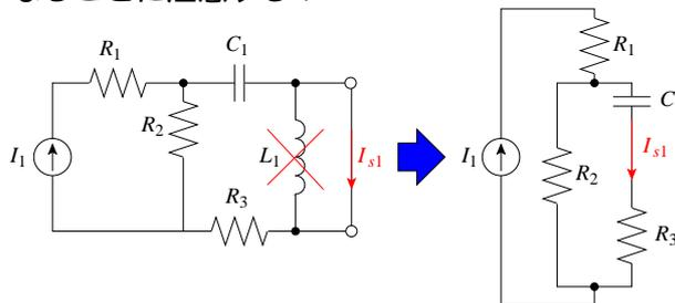
$$I_{s1} = \frac{R_2}{R_2 + \left(R_3 + \frac{1}{j\omega C_1}\right)} I_1 = \frac{j\omega C_1 R_2 I_1}{1 + j\omega C_1 (R_2 + R_3)}$$
