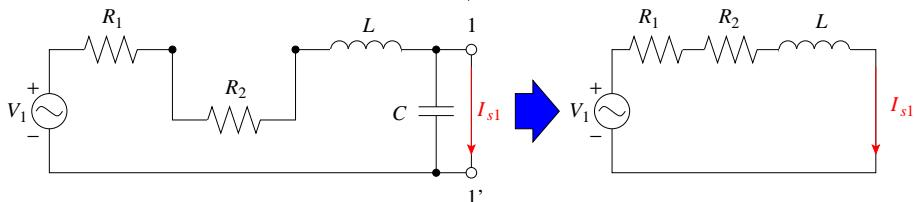
$$I_{s1} = \frac{V_1}{R_1 + R_2 + j\omega L} = \frac{2}{1+4+j5} = \frac{2}{5(1+j)} = \frac{1-j}{5} \text{ A}$$
