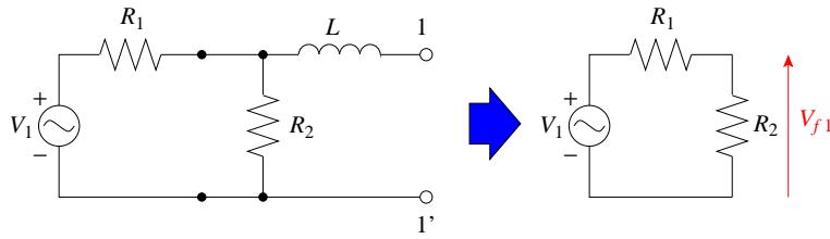
$$V_{f1} = \frac{R_2}{R_1 + R_2} V_1 = \frac{6}{3+6} \cdot 3 = 2 \text{ V}$$
