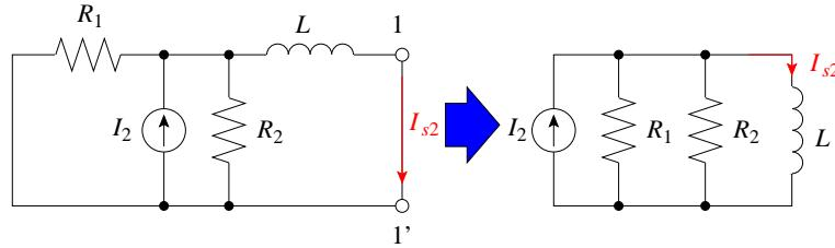
$$I_{s2} = \frac{\frac{1}{j\omega L}}{\frac{1}{R_1} + \frac{1}{R_2} + \frac{1}{j\omega L}} I_2 = \frac{\frac{1}{j2}}{\frac{1}{3} + \frac{1}{6} + \frac{1}{j2}} = \frac{-j3}{2 + 1 - j3} = \frac{-j}{1 - j} = \frac{1-j}{2} \text{ A}$$
