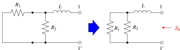
$$Z_0 = (R_1 // R_2) + j\omega L = \frac{R_1 R_2}{R_1 + R_2} + j\omega L = \frac{3 \cdot 6}{3 + 6} + j2 = 2(1 + j) \Omega$$
