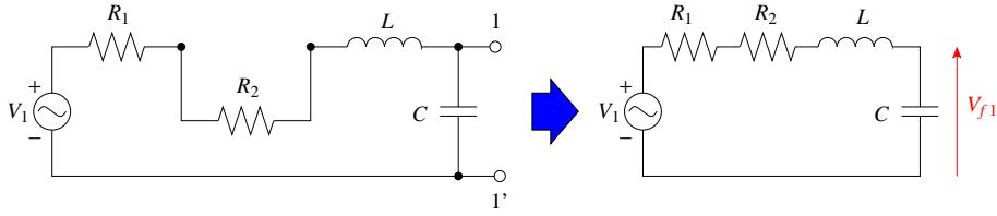
$$V_{f1} = \frac{\frac{1}{j\omega C}}{R_1 + R_2 + j\omega L + \frac{1}{j\omega C}} V_1 = \frac{-j5}{1 + 4 + j5 - j5} \cdot 2 = -j2 \text{ V}$$
