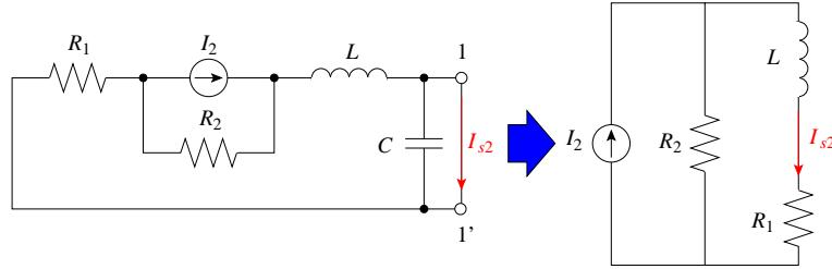
$$I_{s2} = \frac{R_2}{R_2 + (R_1 + j\omega L)} I_2 = \frac{4}{5(1+j)} \cdot 2 = \frac{4(1-j)}{5} \text{ A}$$
