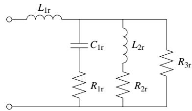
$$R_{1r} = \frac{R_0^2}{R_1}, \quad R_{2r} = \frac{R_0^2}{R_2}, \quad R_{3r} = \frac{R_0^2}{R_3}, \quad L_{1r} = C_1 R_0^2, \quad L_{2r} = C_2 R_0^2, \quad C_{1r} = \frac{L_1}{R_0^2}$$
