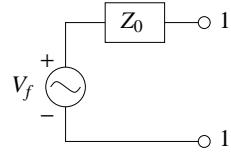
$$Z_0 = \frac{1}{Y_0} = \left( \frac{R_1 + R_2}{R_1 R_2} + j\omega C \right)^{-1} = \frac{R_1 R_2 \{(R_1 + R_2) - j\omega C R_1 R_2\}}{(R_1 + R_2)^2 + \omega^2 C^2 R_1^2 R_2^2}$$
