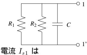
$$Y_0 = \frac{1}{R_1} + \frac{1}{R_2} + j\omega C = \frac{R_1 + R_2}{R_1 R_2} + j\omega C$$
