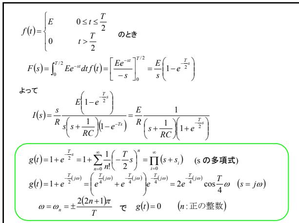
$$I(s) = \frac{E}{R} \frac{1}{\left( s + \frac{1}{RC} \right) \left( 1 + e^{-\frac{T}{2}s} \right)} = \frac{K}{s + \frac{1}{RC}} + \sum_{n=0}^{\infty} \left( \frac{K_n^-}{s - j\omega_n} + \frac{K_n^+}{s + j\omega_n} \right)$$
