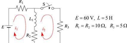
$$t = 0 \text{ で } i_1 = \frac{E}{R_1 + R_2} = \frac{60}{20} = 3 \text{ A}, i_2 = 0 \text{ A}$$
