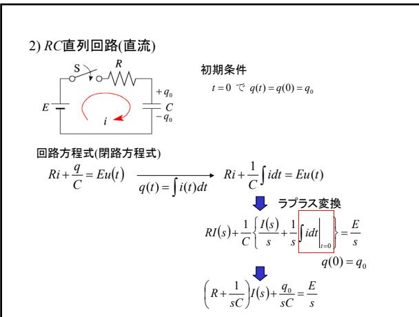
$$I(s) = \frac{CE - q_0}{sCR + 1} = \frac{\frac{1}{R} \left( E - \frac{q_0}{C} \right)}{s + \frac{1}{CR}} \quad \xrightarrow{\text{ラプラス逆変換}} \quad i(t) = \frac{1}{CR} (CE - q_0) e^{-\frac{t}{CR}}$$
