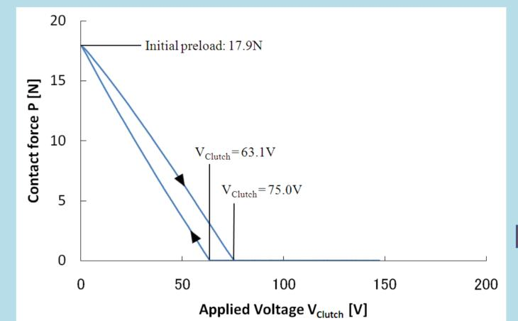
$V_{clutch} = 75.0V$ : The head of the USM was separated from the load cell.  $V_{clutch} = 63.1V$ : The head of the USM was contacted again to the load cell.
