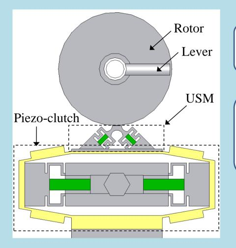
**USM** part : Generate a thrust. Piezo-clutch part : Control a preload.
