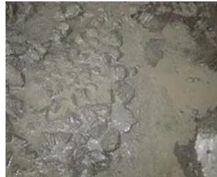
Premature water release leads to bleeding
