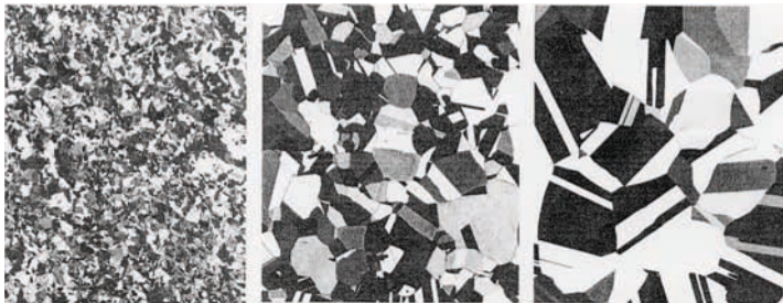
再結晶完了(580°C, 8s) 粒成長(580°C, 15min) 粒成長(700°C, 10min)
