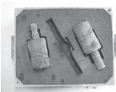
Fig. 4 Frozen mold and frozen core
