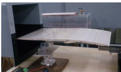
Fig. 5. A flat plate wing with a parabolic rear surface.
