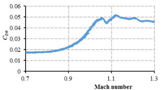
Fig. 4. Parasite drag coefficient at various Mach numbers.
