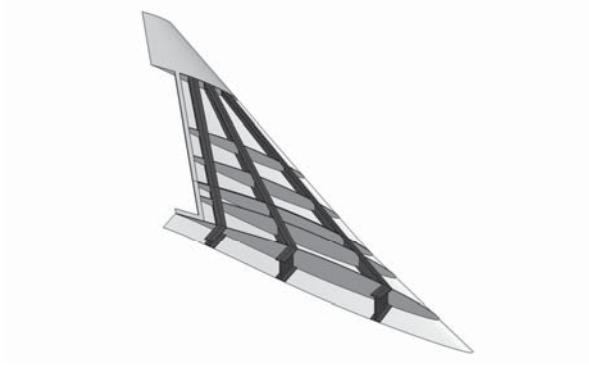
Fig. 2.2. Designed metal structure(2024-T4) of the main wing for the M2007 configuration, where the upper skin is omitted.
